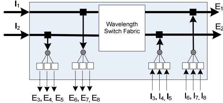
**Figure 6.** A higher degree ROADM with per port add/drop.
