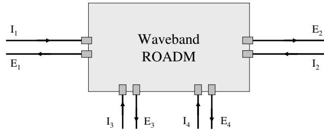
**Figure 3:** ROADM with waveband add/drop ports
