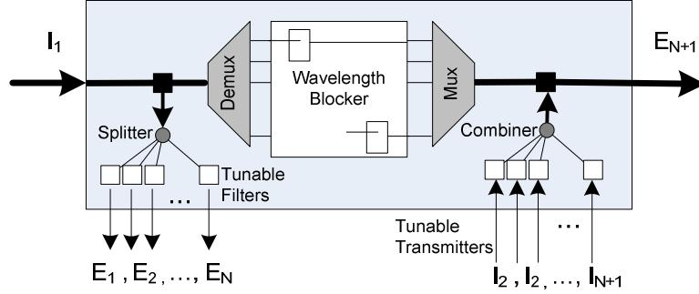
**Figure 2.** A possible implementation of a type II ROADM.
