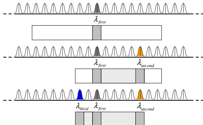
**Figure 5:** The figure shows allocated and available wavelengths, and the waveband tuning constraint after the first, second, and third wavelength has been allocated. The meanings of the
