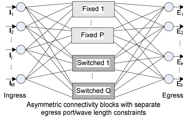
**Figure 11.** General representation of a WSON switch without wavelength converters.
