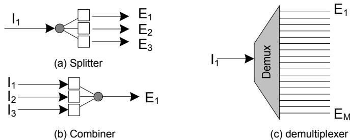
**Figure 8.** Examples of common fixed WSON subsystems.
