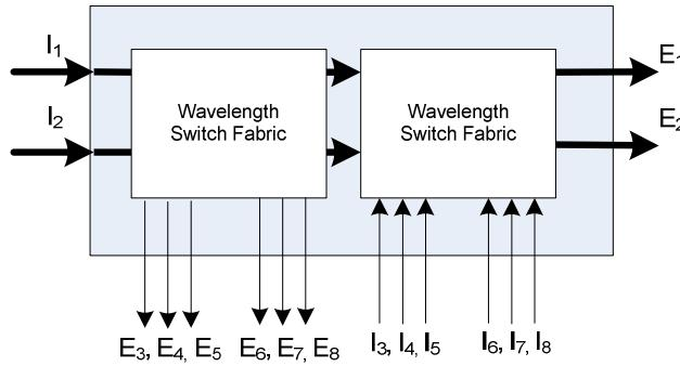
**Figure 7.** A higher degree ROADM with per node add/drop
