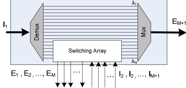
**Figure 9.** A type II ROADM with additional constraints.
