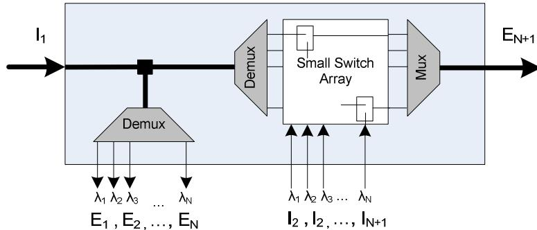
**Figure 1.** One implementation of a type I ROADM.
