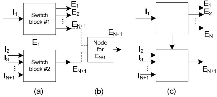
**Figure 13.** Reduced graph representation for our 2-degree ROADM example.
